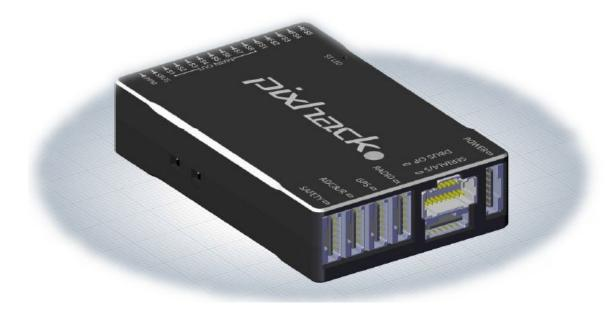
Pixhack, a 32-bit open source hardware flight control, based on Pixhawk hardware architecture platform ,designed and produced by CUAV. As the main architectural hardware the same with pix, so fully compatible with the 3DR APM firmware and pix native firmware.
